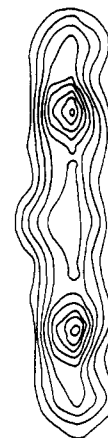
Figure 1. (-1,0,3) section of the difference Fourier map of CuVP 2 S 6 before the introduction of copper atoms in the structure refinement. Three nonequivalent positions clearly show up: Cu1 in the center, Cu2 in the middle (predominant maximum), and Cu3 on the outside. Contour lines: 1.0, 1.5, ..., 5.0 × 10 -6 e/pm 3 .
